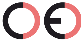
False CE Mark (too far)
